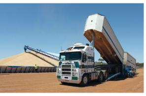
Drive Over Hopper in operation – B-double trailer
