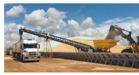
Outloading via BunkerStacker3000 fitted with surge hopper
